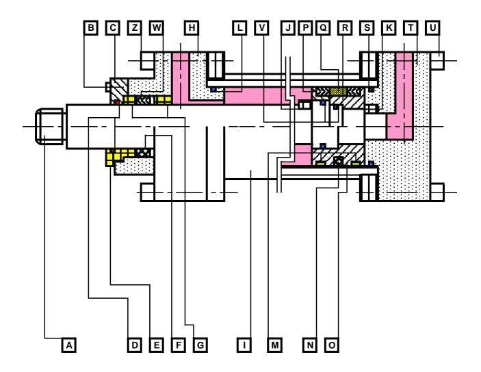
TOP HALF VIEW: version with chevron gasket and with cushioning both sides BOTTOM HALF VIEW: version with low friction gasket and without cushioning
